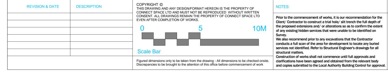
NOTES: Prior to the commencement of works, it is our recommendation for the Client/ Contractor to construct a trial hole/ slit trench the full depth of the proposed extensions and/ or alterations so as to confirm the extent of any existing hidden services that were unable to be identified on We also recommend prior to any excavations that the Contractor conducts a full scan of the area for development to locate any buried services not identified. Refer to Structural Engineer's drawings for all
